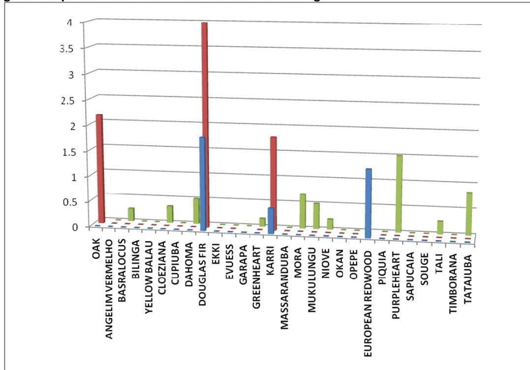
**Figure 7: The comparative performance of the candidate timbers against attack by shipworm expressed as a mean visual assessment rating**
