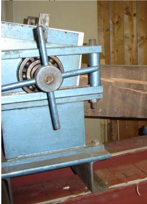
**Figure 4: Support Secured Beneath I-Beam**
