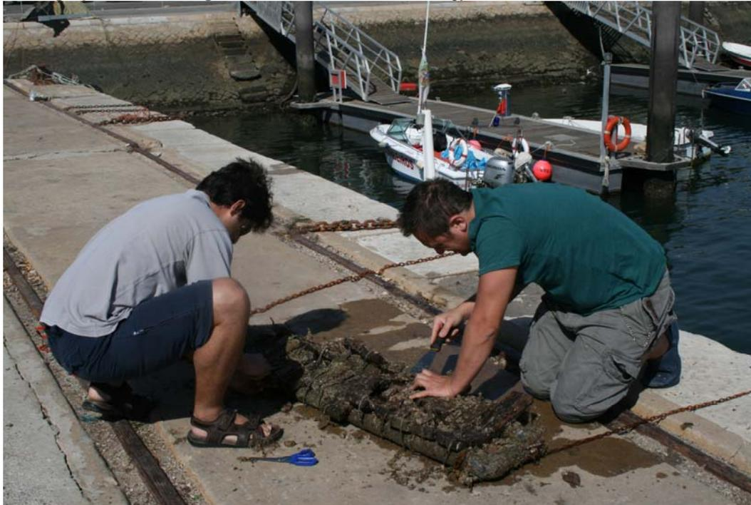
**Photograph 17: Typical fouling.** Note that removal of the barnacles leaves behind a calcareous deposit (arrowed) that has to be removed prior to assessment for attack by gribble and assessment using X ray photography. *TRADA Technology*
