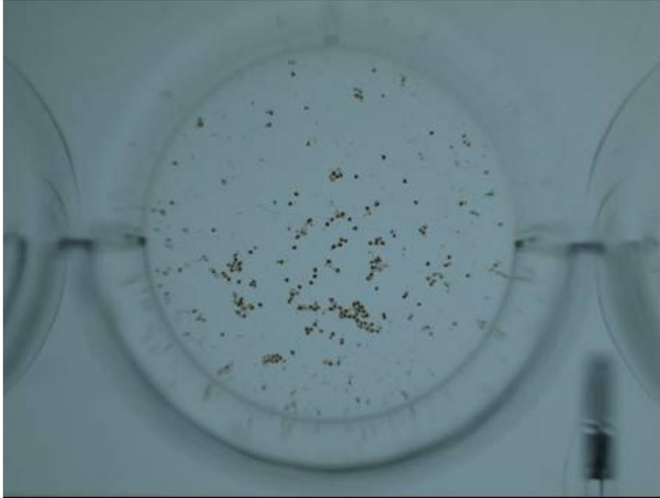
**Photograph 7: European redwood sapwood and comparatively high feeding rate expressed as faecal pellet production.** *Courtesy S Cragg: University of Portsmouth*
