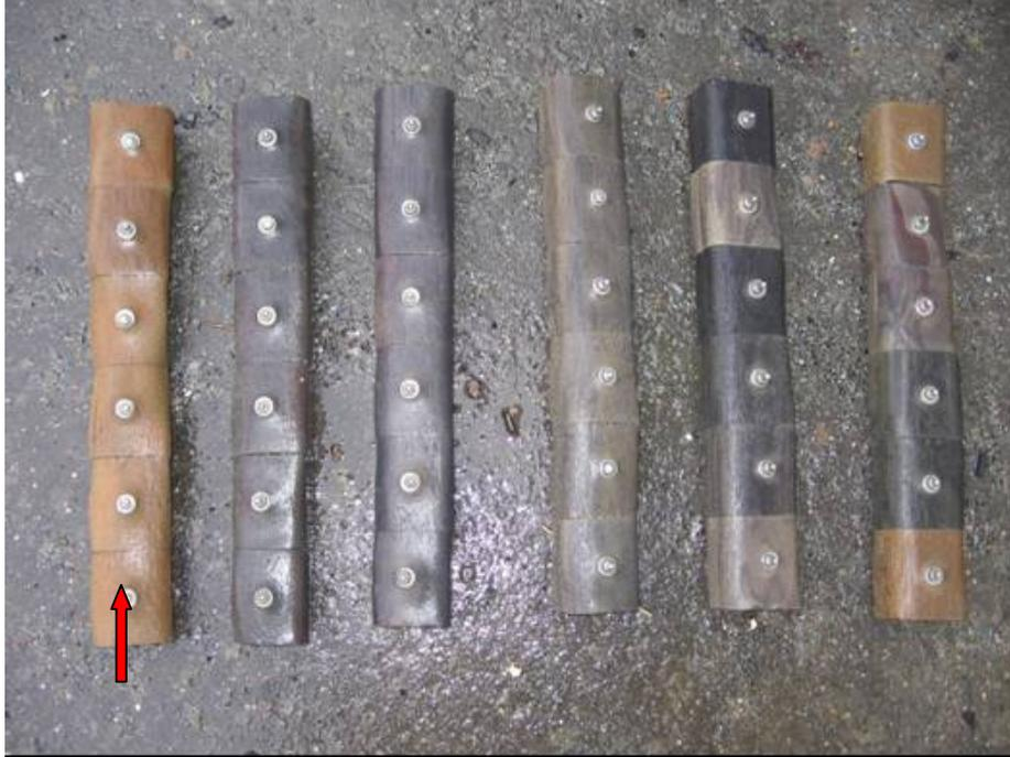
**Photograph 12: Test rack supporting greenheart after 160,000 cycles.** *Courtesy Gervais Sawyer*
