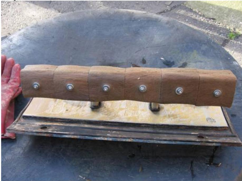
**Photograph 13: Cold forging of the steel caused by abrasion of the shingle. Courtesy Gervais Sawyer**
