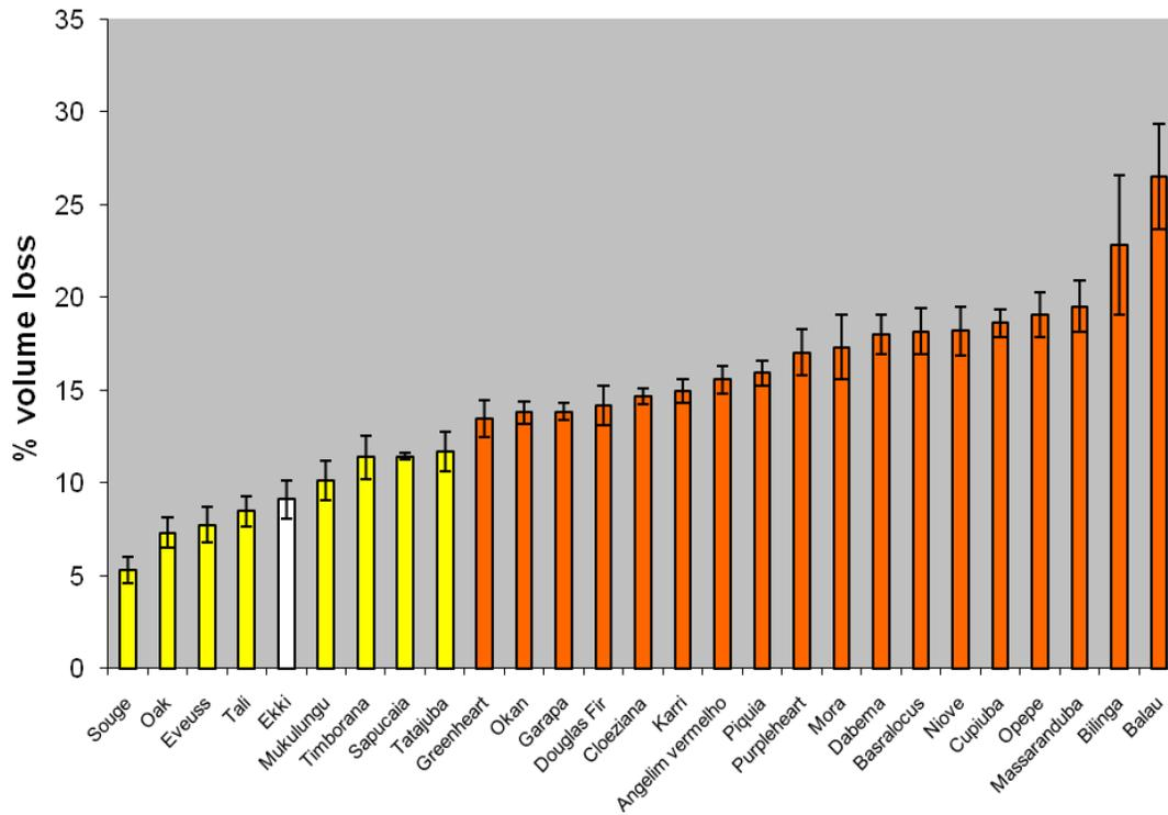
**Figure 4: Average volume loss after 160,000 cycles for the candidate species compared to Greenheart.**
