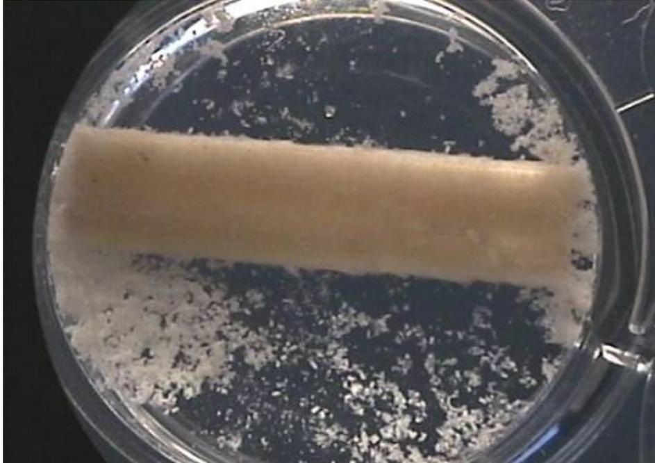
**Photograph 8: Ekki with dead gribble (arrowed).** Courtesy S Cragg: University of Portsmouth
