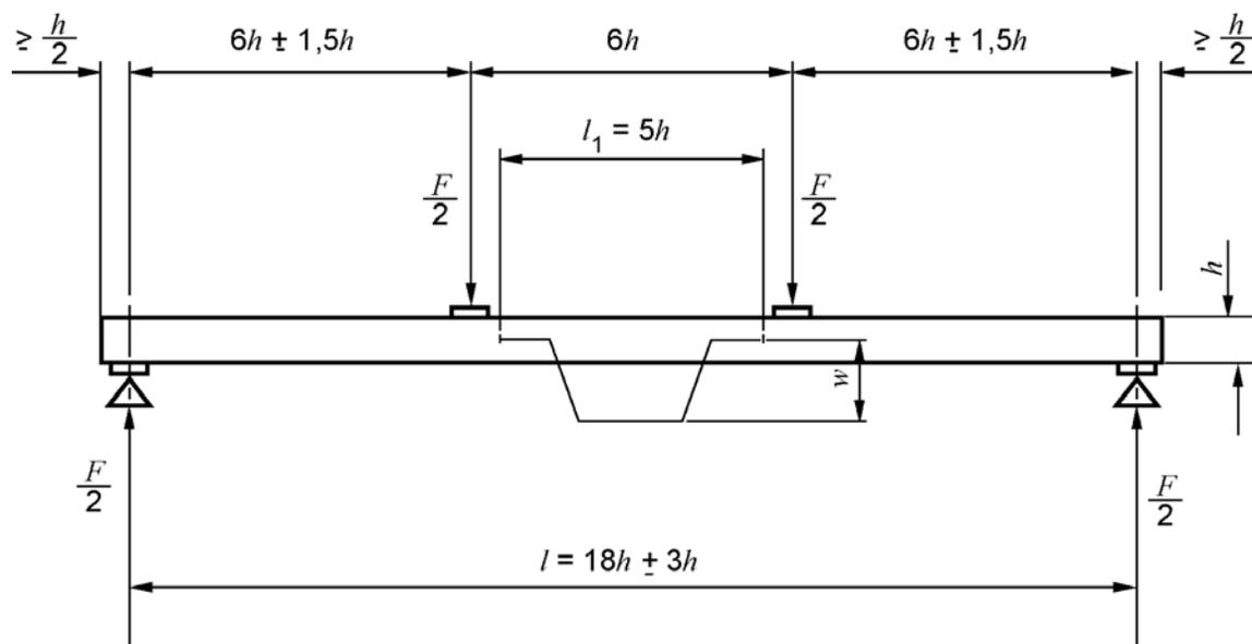
The specimens were symmetrically loaded in bending on simple supports at two points over a span of 18 times the depth. The permitted variation in the overall target span of  $\pm 3h$ , where  $h$  is the depth of the specimen, was not used. The standard does not provide tolerances for the target lengths, although a tolerance of  $\pm 2\text{mm}$  is reasonable.
